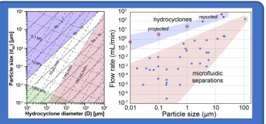
Cyclone scaling enables <100 nm particle isolation
