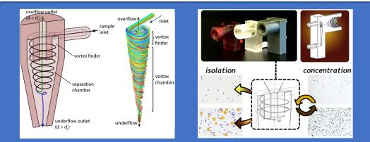
Size-dependent particle trajectories due to inertia, buoyancy, and drag force
